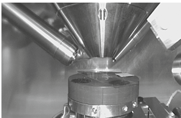
Fig. 2 Mineral wool fibers fixed on polyester foil. The chamber scope image also shows the position of the XTrace's polycapillary optics (right of the microscope pole piece) and the EDS detector (left of the pole piece).
