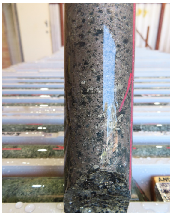
Figure 1: Massive, semi-massive and blebby nickel and copper sulphides in ANDD0003: ~79m downhole
