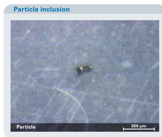
Fig. 4 Inclusion of a small particle in a plastic film
